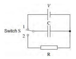
The switch is then moved quickly to position 2, allowing  $\boldsymbol{C}$  to discharge through the fixed
